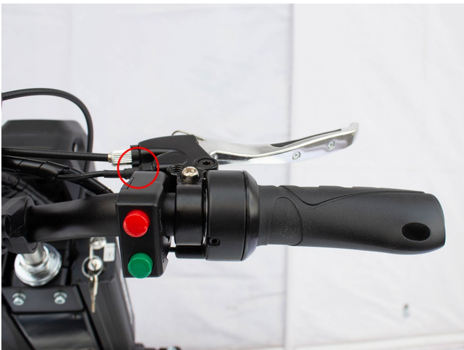
Fig. 42: Brake lever with brake contact and initiation of recuperation (interrupter contact is only connected to the right brake lever.)
