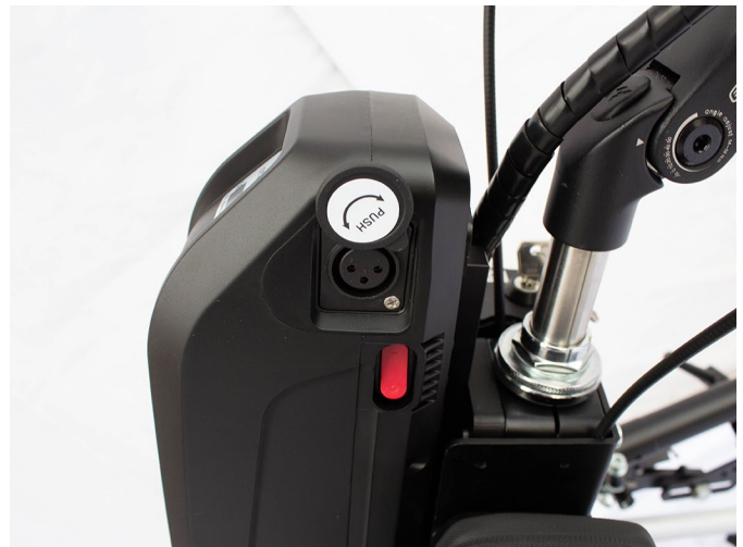
Fig. 33: Switch on the battery
