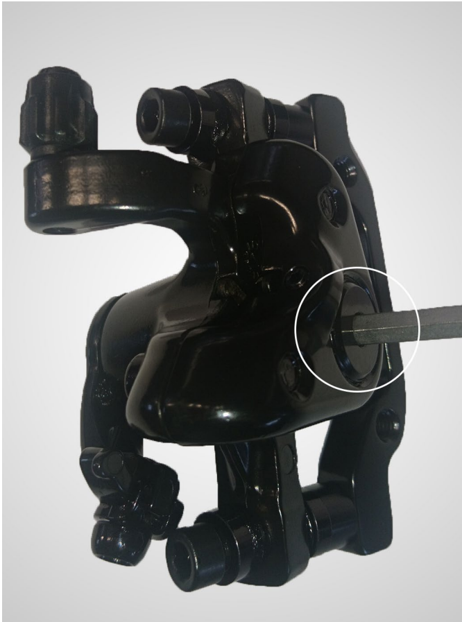
Fig. 48: Loosening the 5 mm brake shoe adjuster
