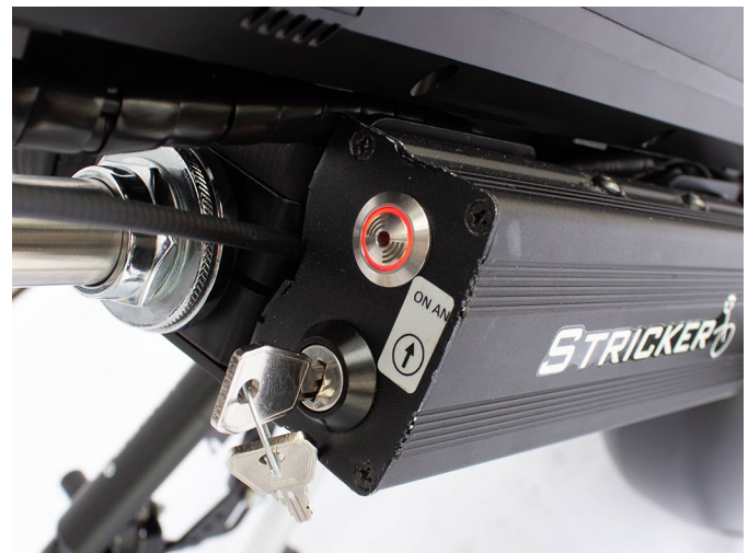
Fig. 41: The reverse light on the control lights up when reverse gear is activated
