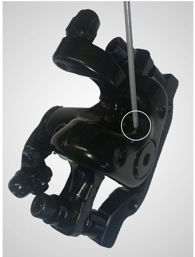
Fig. 47: Loosening the 2 mm grub screw
