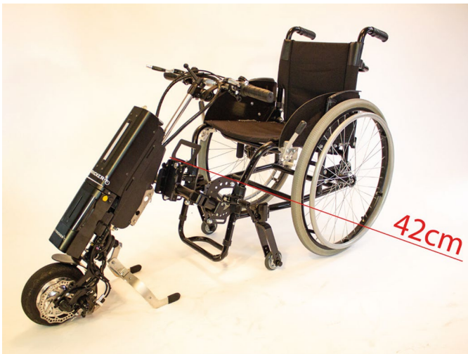
Fig. 13: Adjusting the Lipo Lomo Pico
