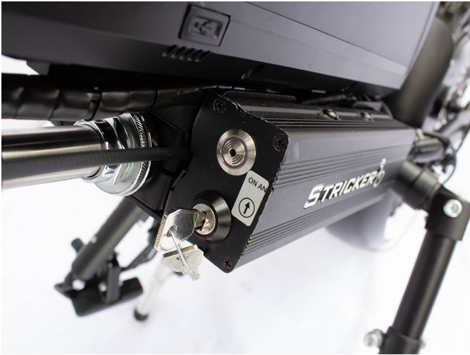
Fig. 34: Key switch on battery and control
