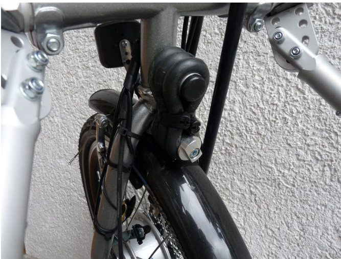
Fig. 43: Steering damper setting
