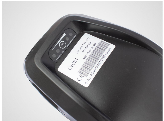
Fig. 32: Battery charge level indicator
