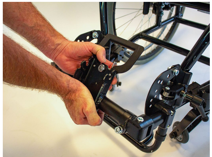
Fig. 18: Coupling plate tilted too much
