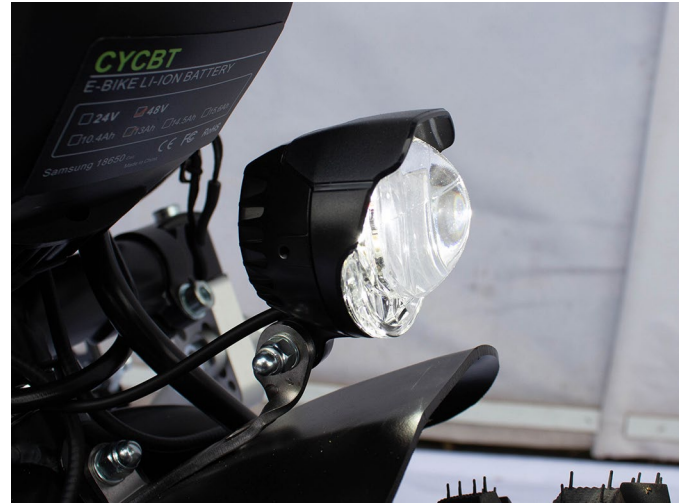
Fig. 40: Adjustment of the inclination of the lamp with integrated horn
