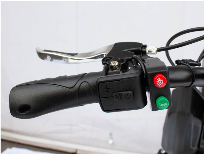
Fig. 35: Control unit on the left handle
