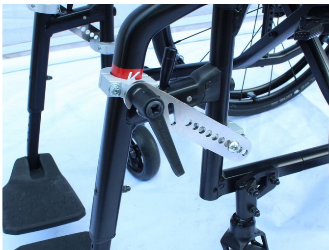
Fig. 5: The pre-mounting fix stabilises the swing-away footrests and enables a stable clamp connection.
